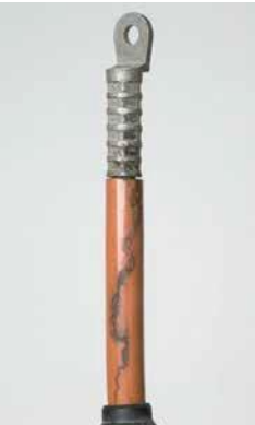
Sample damaged by tracking
